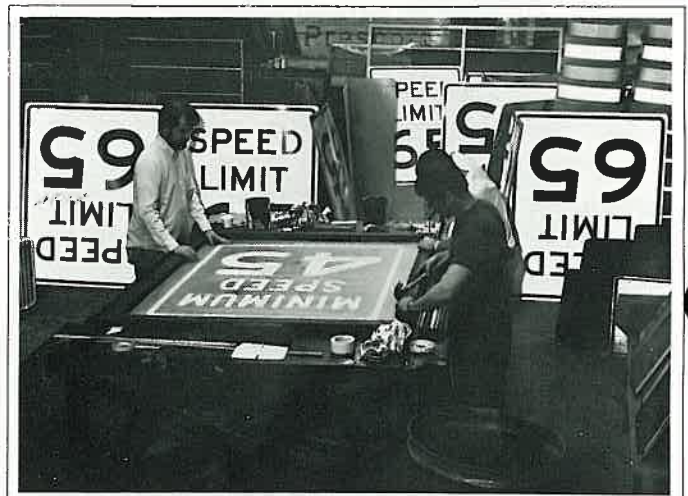
Department sign makers prepare a screen for the new "Minimum Speed" sign.
